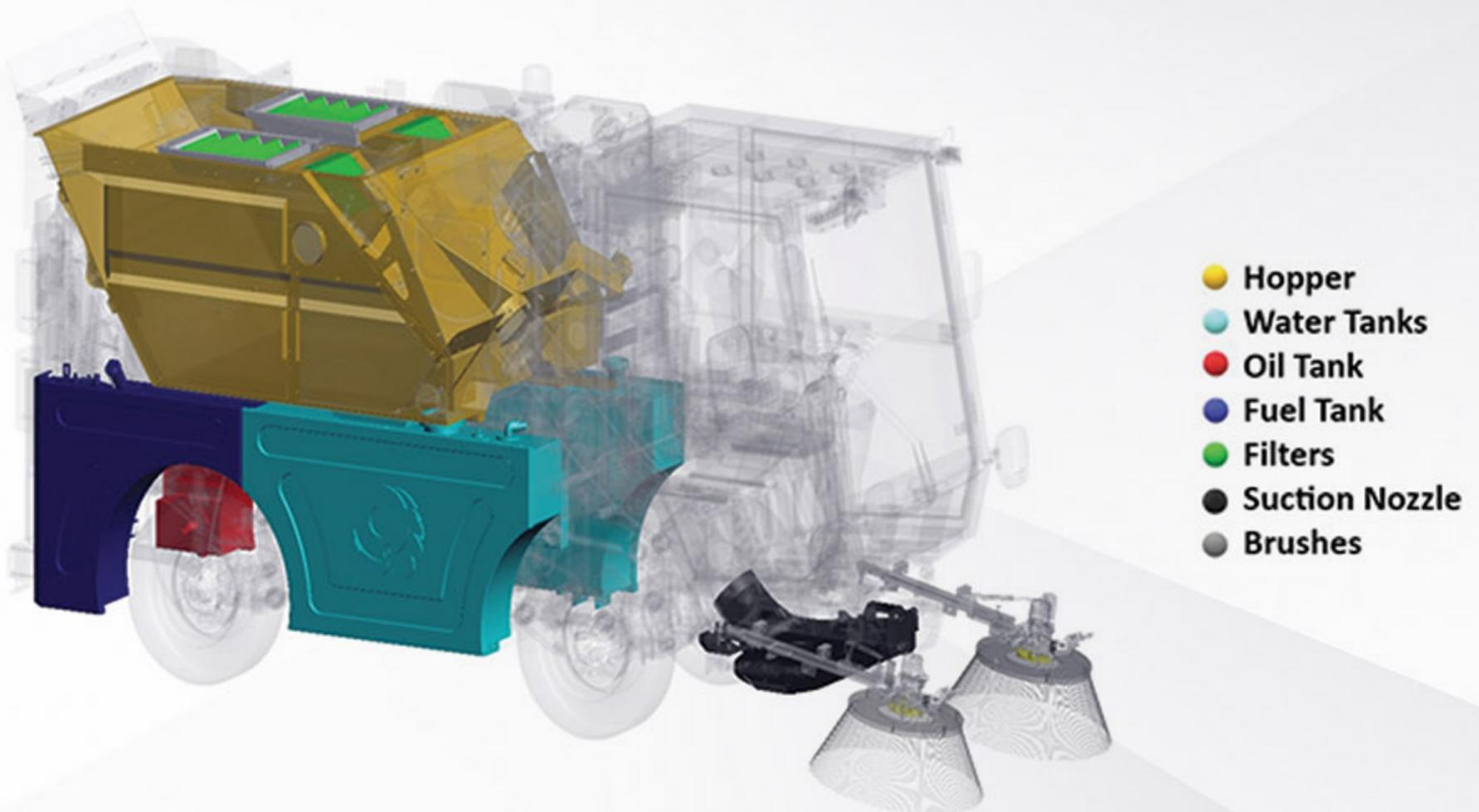
**Hopper:** 2+ m<sup>3</sup> hopper which is constructed from aluminium metal permits an increased radius of action and maximum debris collection; and it provides maximum comfort for the driver for long working days.
