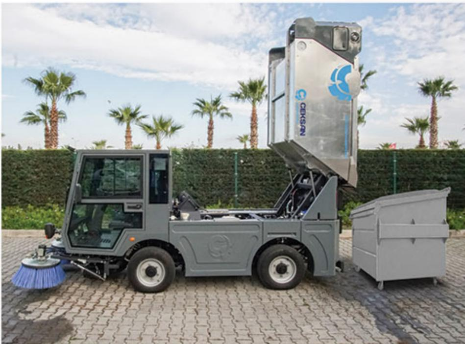
**Unloading:** CityMouse is equipped with a high-dump system for emptying the container. The hopper lid opens hydraulically. A sturdy rubber gasket guarantees water-proof sealing during sweeping operations and prevents external air from being drawn in.
