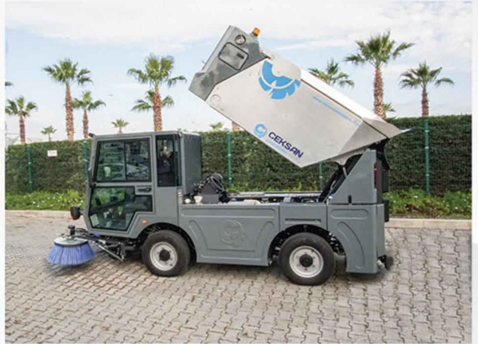
**Dust Suppression and Water Recirculation System:** Proper use of water is essential not only for dust suppression but also sweeping performance and longevity of sweeper components. Both brushes have stainless water jets to prevent dust while working. Waste is humidified at correct points throughout suction nozzle. Water level can be monitored on control unit.
