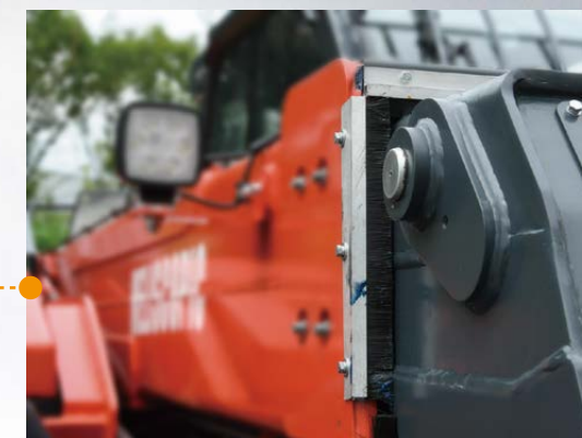
Brushes inside the boom to prevent the particles and dust during work
