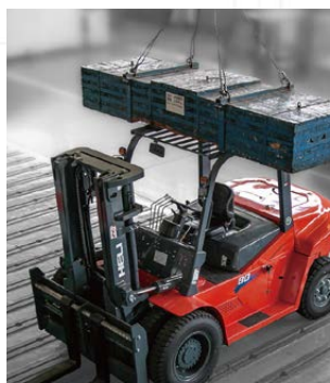
Impact test of overhead guard
